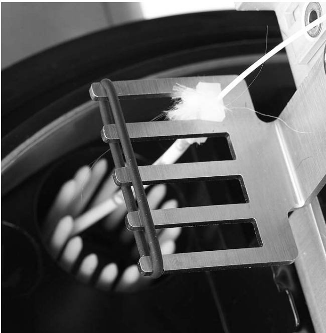
3.7 Pull back the cable and install the mini KTU in the holder. Secure with the O-ring.
